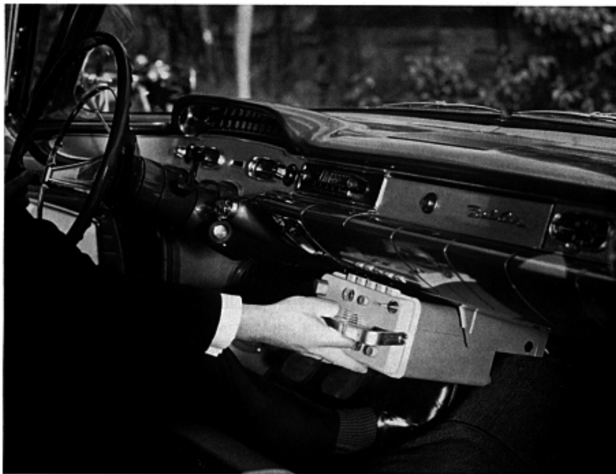
Fig.1. The radio code paging receiver as fitted under the dashboard of a car.
